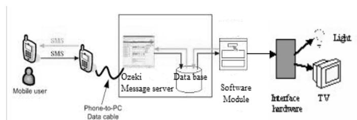
Figure 3 – Design of Remotely Controlled System
