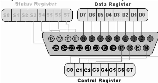
Figure 1- Pin outs of DB25
