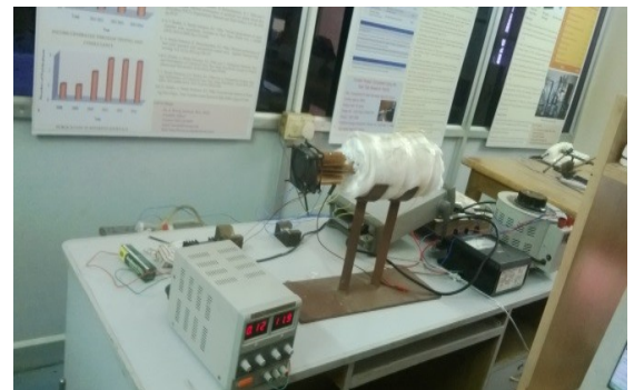
Experimental setup of mould and heat pipe
