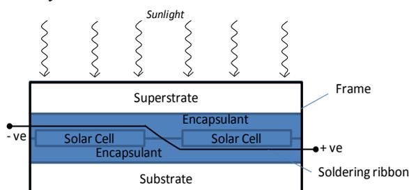
Figure2: Schematic cross section of a solar panel assembly. [8]
