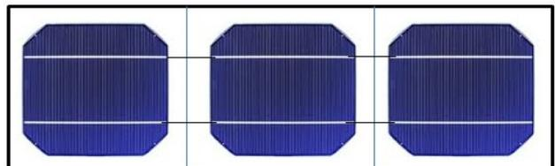
Figure1: solar cells convert in series. [9]
