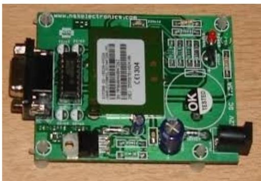
Fig 4: GSM Modem
