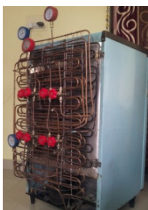
Fig 1 Proposed System with condenser coil lengths of 9.14m, 9.45m, 9.75m & 10.06m.
