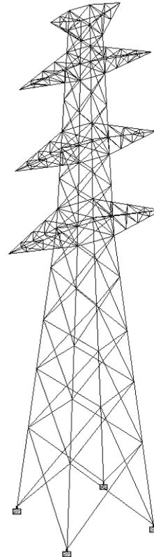
Fig 1. Isometric view of 472 bar Transmission Line Tower
