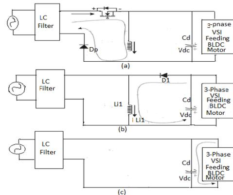
Fig. 2. Operation of the proposed converter in numerous modes (a)–(c) for a positive half cycle of supply voltage and (d) the associated waveforms. (a) Mode I. (b) Mode II. (c) Mode III.
