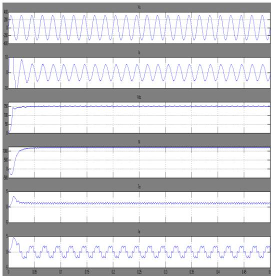
Fig. Steady-state performance of the proposed BLDC motor drive at rated conditions.
