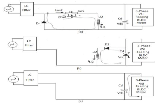
Fig. 3. Operation of the proposed converter in different modes (a)–(c) for a negative half cycle of supply voltage and (d) the associated waveforms. (a) Mode I. (b) Mode II. (c) Mode III.
