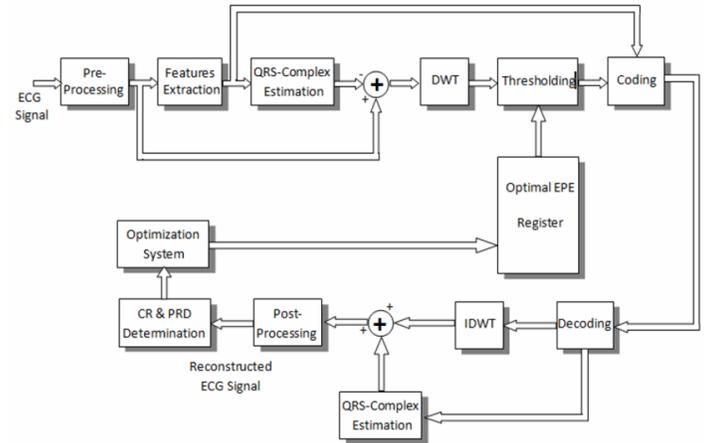
Figure 2 Block diagram of ECG compression[1]
