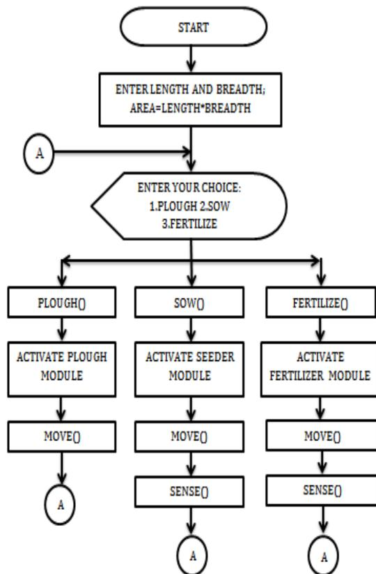
Fig 3.System Algorithm
