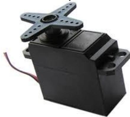
3.7 Kg torque servo motors are used to bear the weight of the robot. The servos on central plate of chassis help the robot lift up the legs. The ultrasonic sensors on the robot give the distance between any obstacle in front.
