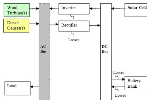
Fig 2.3 Wind-Diesel and PV hybrid system schematic
