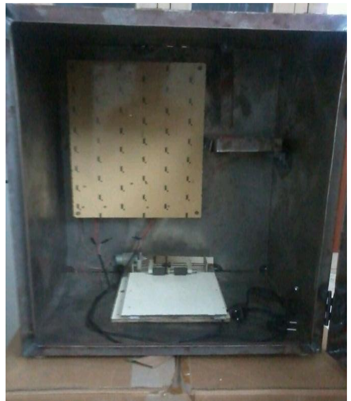
Fig. 14 Interior of the automatic paper vending machine back side
