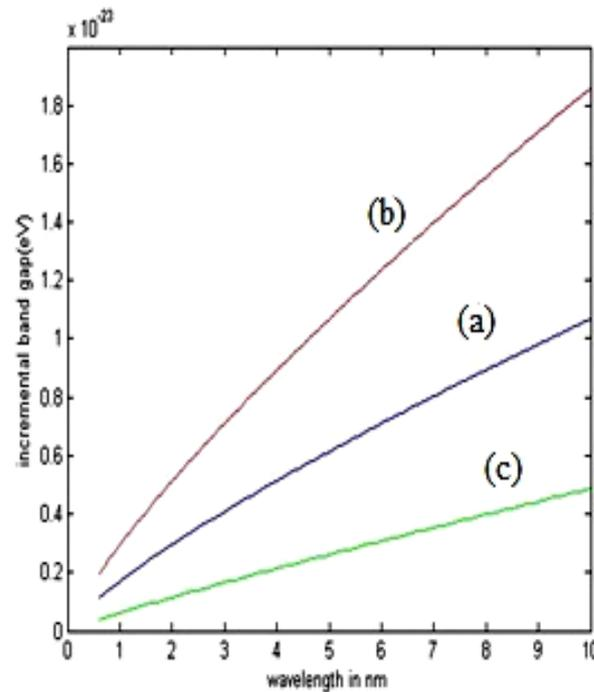
Figure 1 & 2 : (a) and (b) represent the variations according to perturbed three- and two-band models of Kane respectively. The curve (c) represents the same variation in  $n\text{-In}_{1-x}\text{Ga}_x\text{As}_y\text{P}_{1-y}$  in accordance with the perturbed parabolic energy bands
