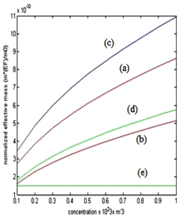
Figure 3 & 4: EMM  $n\text{-In}_{1-x}\text{Ga}_x\text{As}_y\text{P}_{1-y}$  in the presence of light waves in which the curves (a) and (c) represent the three- and two-band models of Kane respectively. The curves (b) and (d) exhibit the same variation in the absence of external photo-excitation. The curve (e) represents the parabolic energy band model both in the presence and in the absence of the external photo-excitation.
