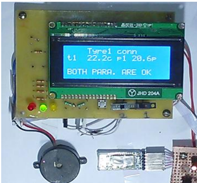
Figure 6: Display of LCD and LED is on for temperature and pressure of tire
