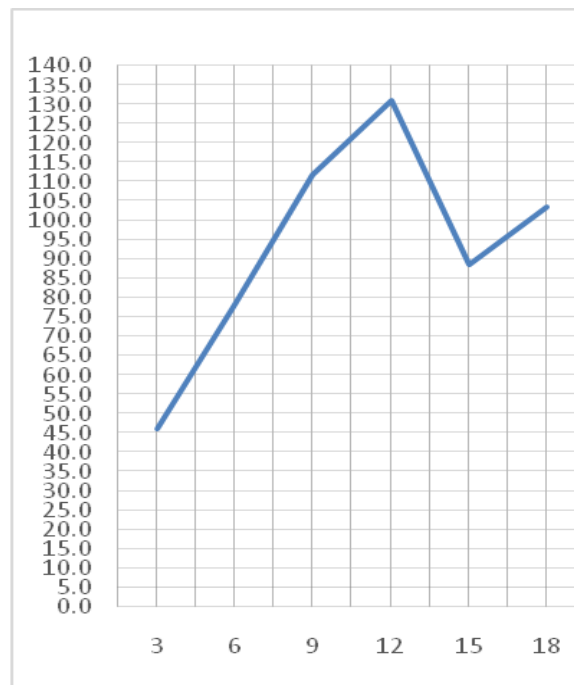
Fig no .3. Premonsoon graph of resistivity (on y axis) Vs depth on (x axis) for point .D
