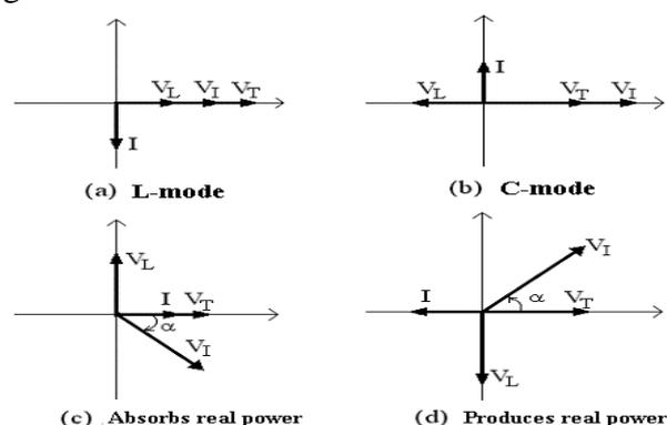
Fig 4.1: Operation of STATCOM
