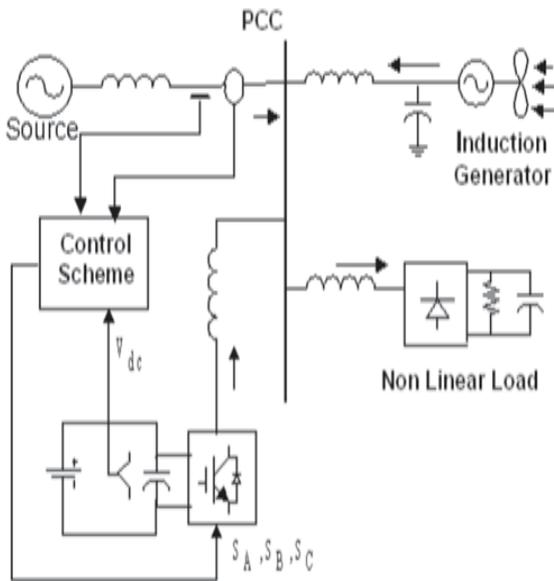
Fig 5: Simulated Circuit Block Diagram.
