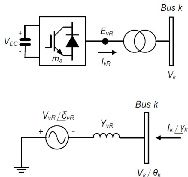
Fig 3.1: STATCOM scheme with equivalent representation.
