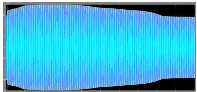
Fig 6.1: Current at coupling point without STATCOM.
