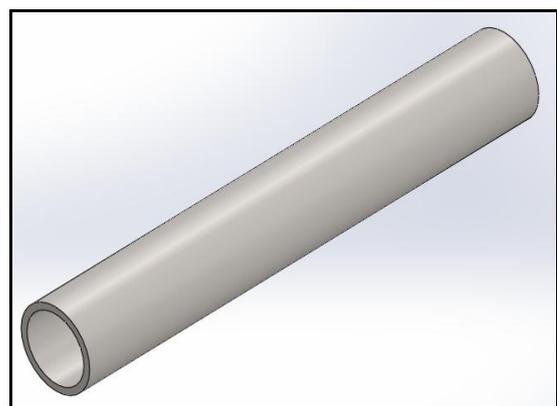
Fig.5 – GI Pipe for Exhaust Outlet
