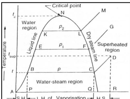
Fig.2 Temperature-Total heat graph during steam formation
