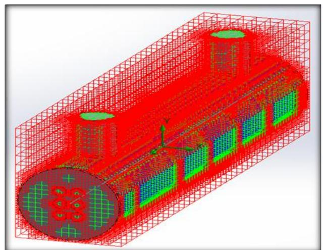
Fig. 7 Meshing of Rectangular CS assembly
