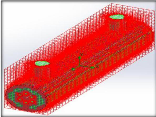
Fig. 8 Meshing of Round CS Assembly
