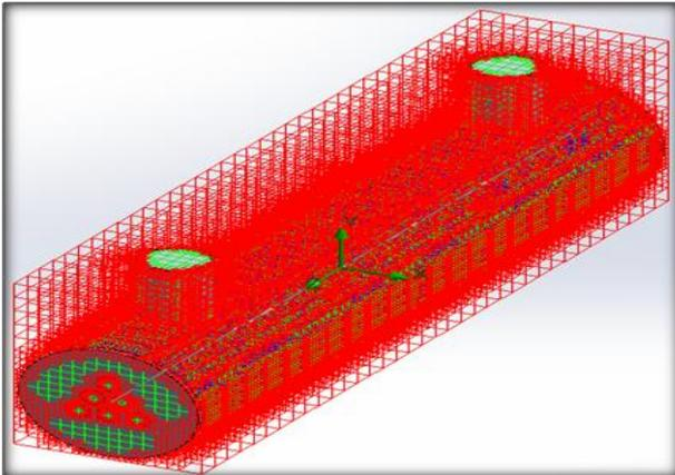
Fig. 9 Meshing of Triangle CS Assembly
