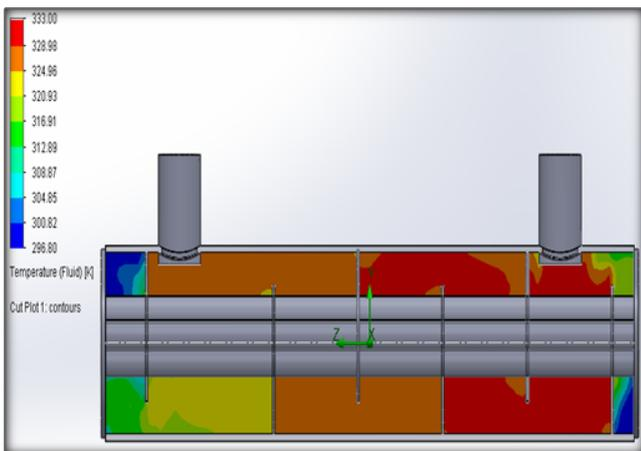
Fig. 15 Temperature Cut Plot (Triangle)
