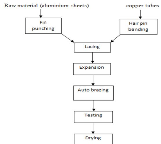
Fig.4.1: flow chart of the coil shop.
