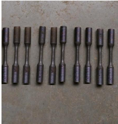
Fig. 5 Tensile specimens of ADI held at different austempering durations.
