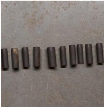
Fig. 6 Hardness specimens held at different austempering duration
