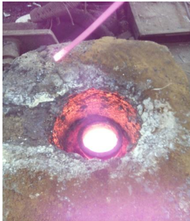
Fig. 2 Preparation of IS500/7 ductile iron by melt
