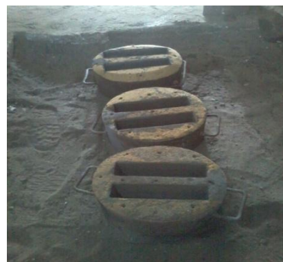
Fig.1 Sand Moulds as per ASTM A897
