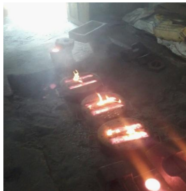
Fig. 3 Pouring of IS 500/7 ductile iron molten metal
