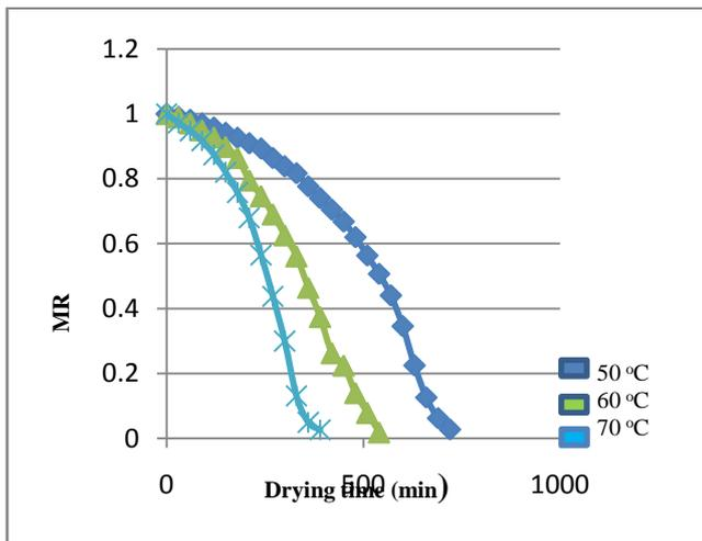
Fig. 3.2 Drying time Vs moisture ratio (MR) at different temperatures
