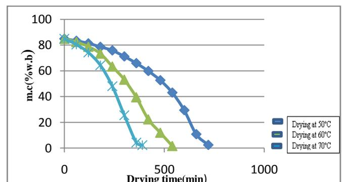
Fig. 3.1 Reduction in moisture content with drying time at different tray temperatures during vacuum drying.
