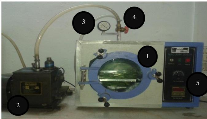
1.Drying Chamber 2. Vacuum pump 3. Vacuum gauge
