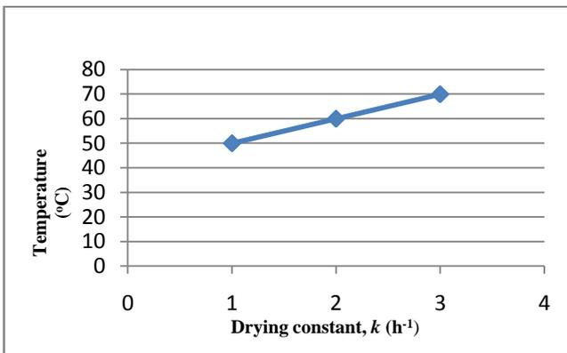
Fig. 3.4 Effect of drying temperature on drying constant ( $k$ ) in Page model
