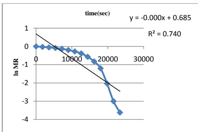
Fig. 3.5  $\ln(MR)$  Vs drying time  $t$  at 70 °C
