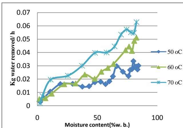
Fig. 3.3 Drying rate Vs moisture content at different drying temperatures
