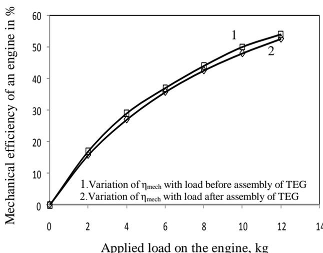
Fig. 6 Variation of mechanical efficiency with applied load
