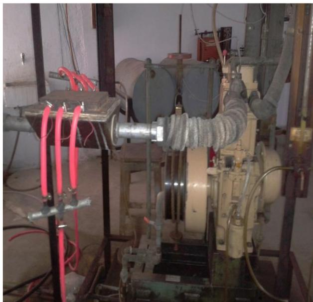
Fig. 4 Assembly of TEG to a Compression Ignition engine.
