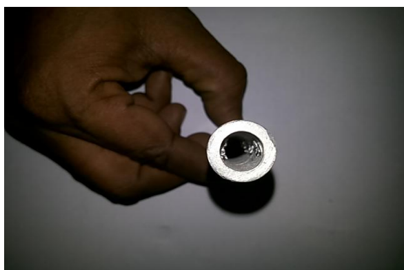
Fig. 5 Perforated Pin Fin used for the purpose
