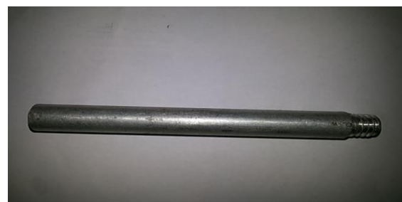
Fig. 4 Solid Pin fin used for the purpose
