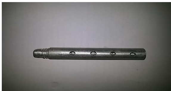
Fig. 5 Perforated Pin Fin used for the purpose
