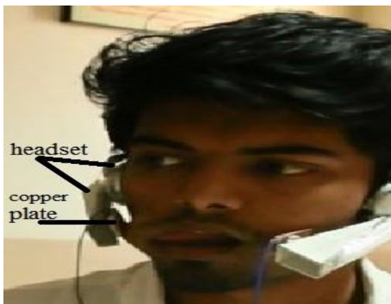
Figure 1: Headgear Assembly (The touch of the cheek is detected by the copper plate due to the movement of the tongue)
