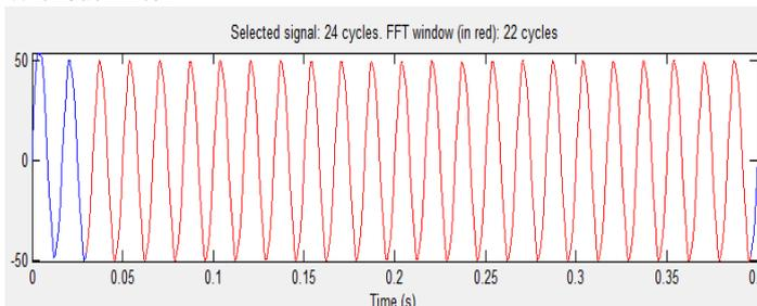
Fig -16(c): Source Voltage Waveform in Phase-a With Hybrid Filter
