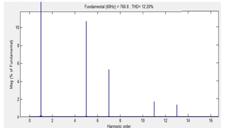
Fig -15(b): THD of Source Current Waveform in Phase-a Without Filter
