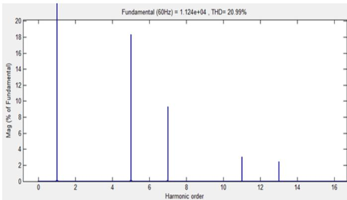
Fig -15(d): THD Spectrum of Source Voltage Waveform in Phase-a Without Filter
