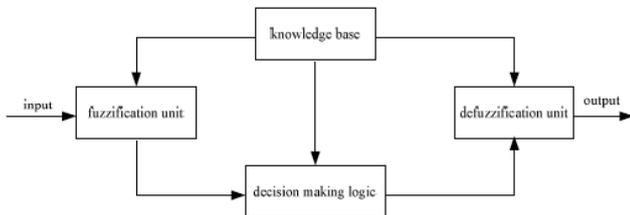
Fig -8: Structure of Fuzzy Logic Controller
