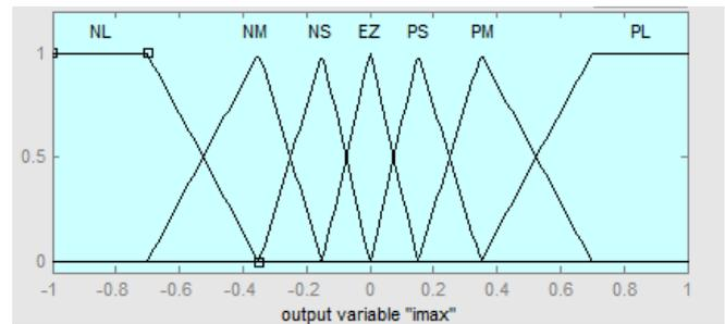
Fig -10(c): Output Membership Function (Peak Supply Current  $i_{max}$ )
