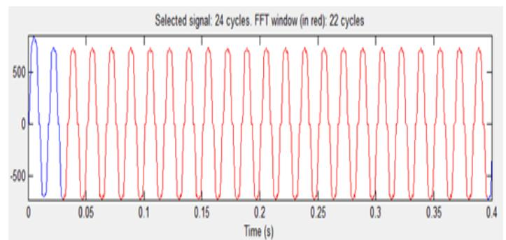
Fig -15(a): Source Current Waveform in Phase-a Without Filter
