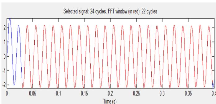
Fig -16(a): Source Current Waveform in Phase-a With Hybrid Filter
