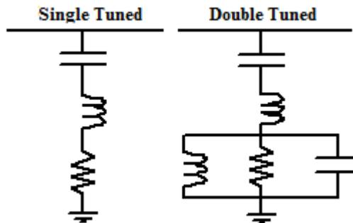
Fig -3: Single and Double Tuned Passive Filters
