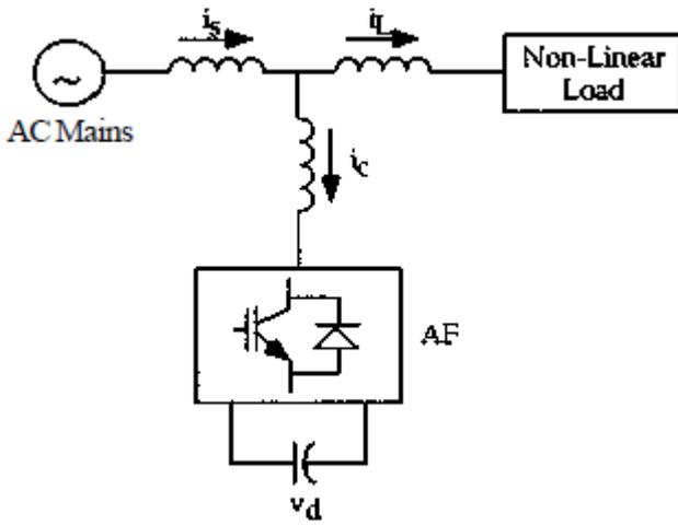
Fig -4: Shunt Active Filter
