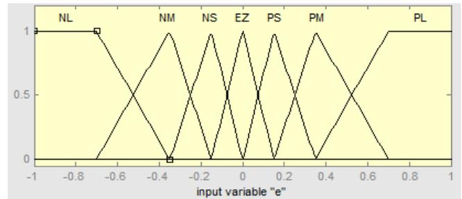
Fig -10(a): Input Membership Function (Error e)
