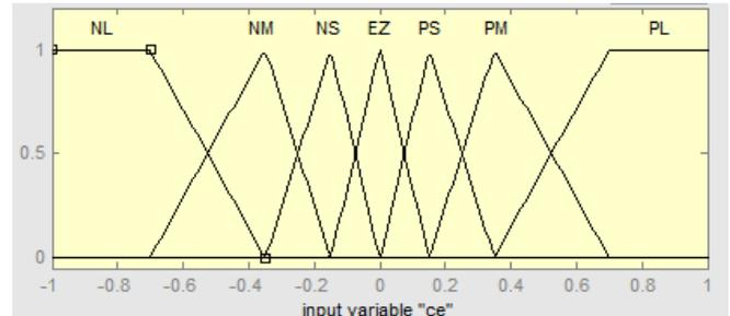
Fig -10(b): Input Membership Function (Change of Error ce)
