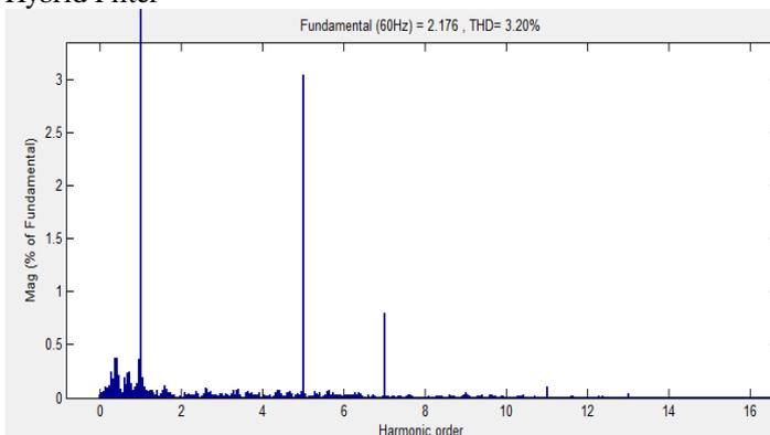
Fig -16(b): THD of Source Current Waveform in Phase-a Without Filter
