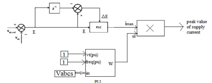
Fig -11: Generation of Reference Compensating Current using Fuzzy Logic Controller
