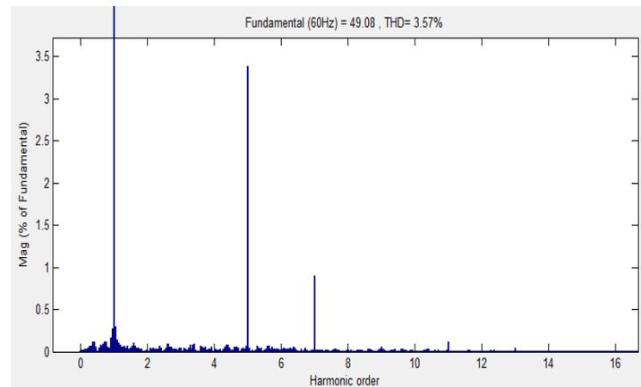
Fig -16(d): THD Spectrum of Source Voltage Waveform in Phase-a With Hybrid Filter.
