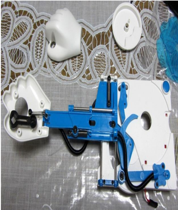
Fig. Components of Auto Pen Writer [5]
