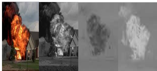
Figure 4: Different channels of YCbCr image, (a) Original frame, (b) Y color channel, (c) Cb color channel, (d) Cr color channel.
