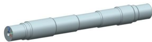
Fig.8. The 3D model of Rail wheel axle (isometric view)
