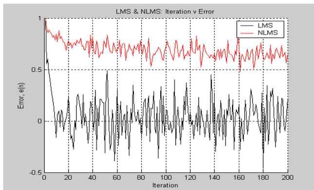
Fig 4. Error convergence performed by LMS and NLMS
