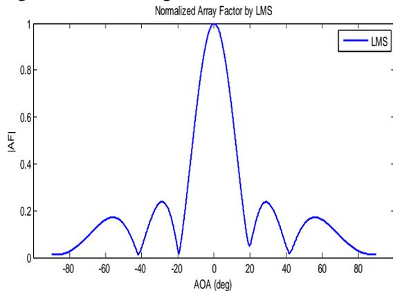
Fig.7. Antenna loading to interference when  $\theta = 0^0$
