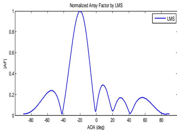
Fig.8. Antenna loading to interference when  $\theta = -20^0$
