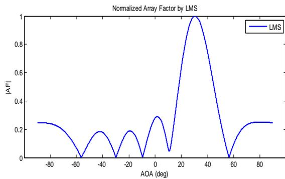
Fig.6. Antenna loading to interference when  $\theta = 30^0$
