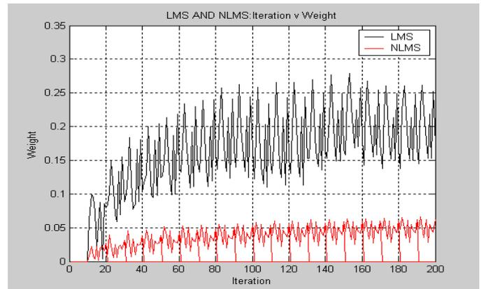
Fig 5. Weight vector convergence performed by LMS and NLMS
