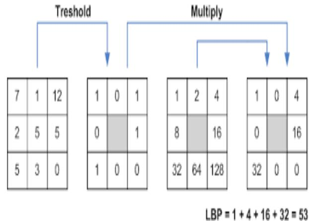
Fig. 3 Calculating the Original LBP Code And A Contrast Measure.
