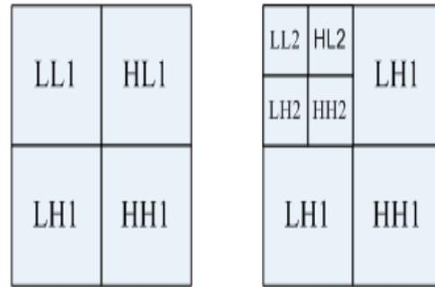
Fig. 2 Image Decomposition (a) One Layer (b) Two Layer
