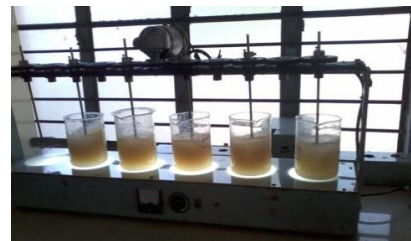
Figure 3 Schematic view of conventional jar test apparatus.
