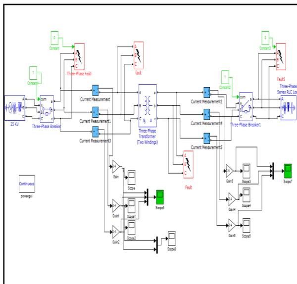
Fig 4 Simulation diagram for transformer fault
