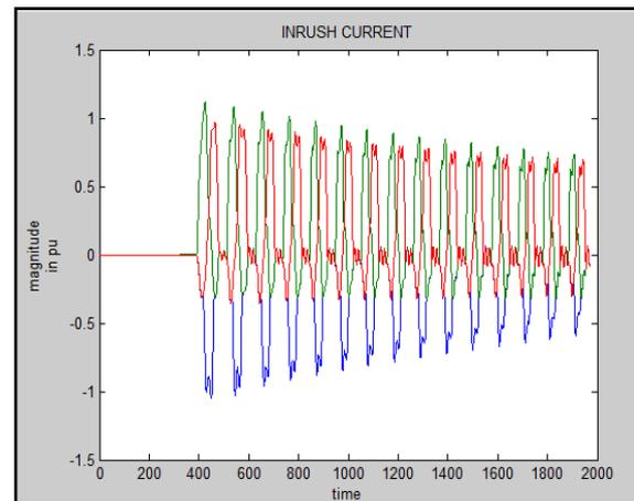
Fig. 6 Waveform for inrush current in transformer
