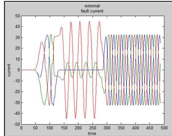
Fig. 5 Waveform for fault current in transformer
