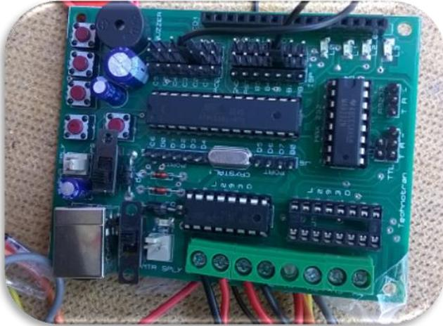
Figure 7: Atmega 8 Robotic Board
