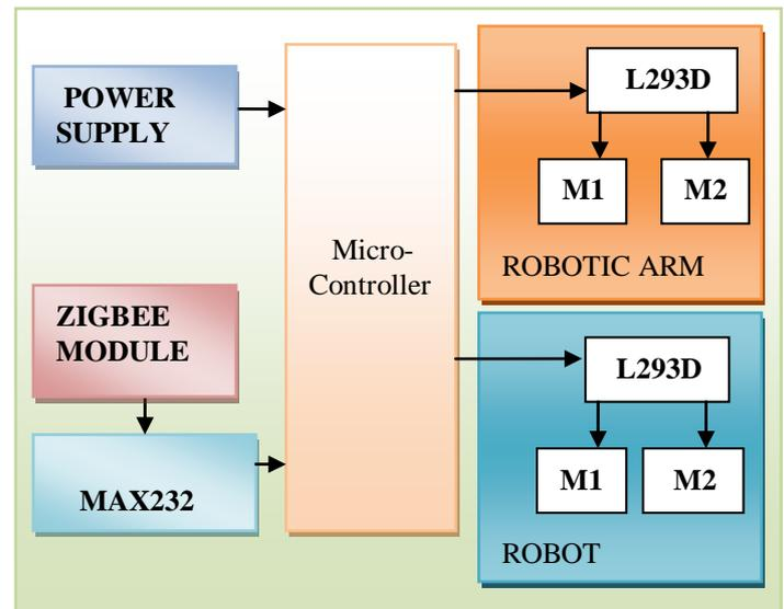
Figure 1: Receiver section
