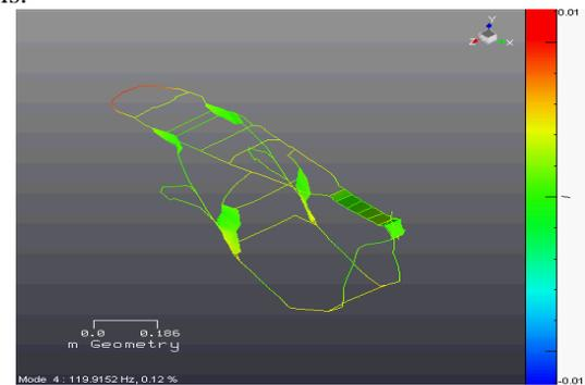
Fig. 3 First Bending Mode
