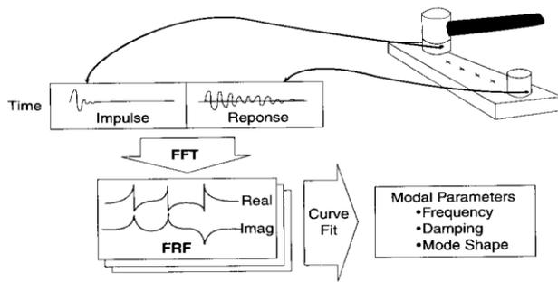
Fig.2. Impact testing
