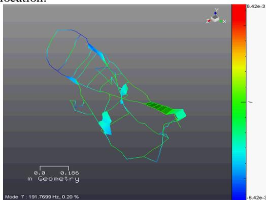
Fig.6. Combine Bending and Twisting Mode
