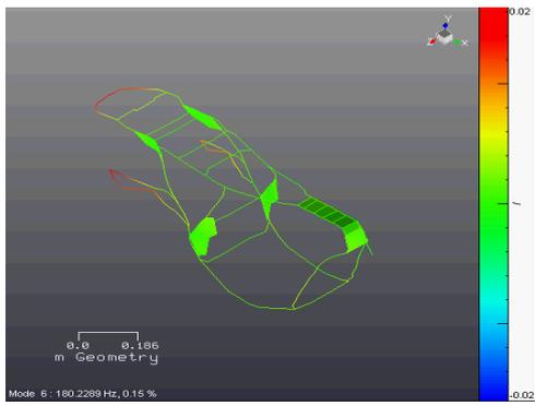
Fig.5 second Bending Mode
