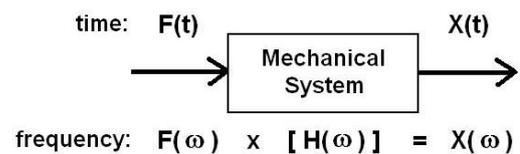
Fig.1 .Block diagram of FRF.
