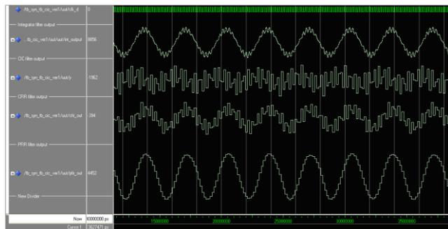
Fig.14 output of CIC decimator filter, CFIR Filter and PFIR filter.
