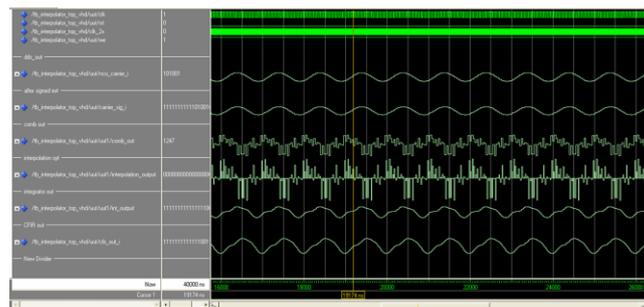
Fig.15 output of CIC interpolation filter.
