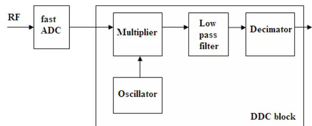
Fig.1 Theoretical DDC Block Diagram
