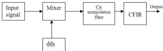
Fig. 12 DUC block diagram using CIC Filters
