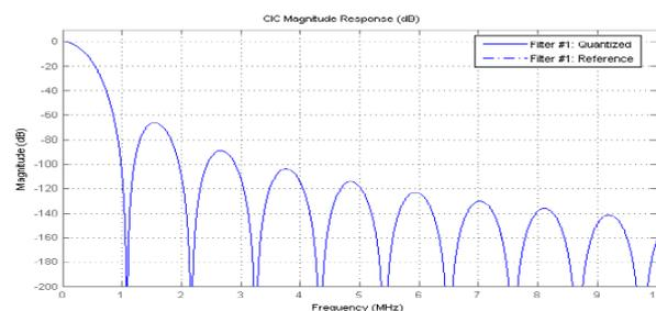
Fig.10 compensation filters response
