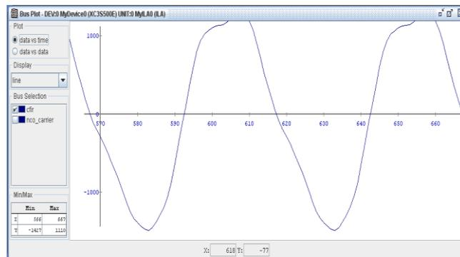
Fig.17 CFIR output of DUC.
