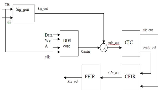
Fig. 7 DDC block diagram using CIC Filters
