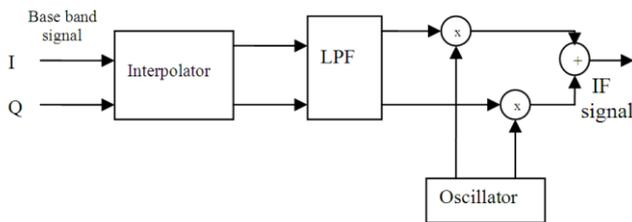
Fig.2 Theoretical DUC Block Diagram
