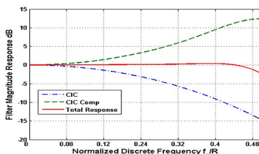
Fig.11 Response after using the CFIR Filter
