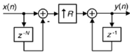
Fig.6 CIC interpolation Filter
