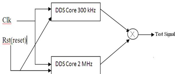
Fig.8 Test signal generator using two DDS cores
