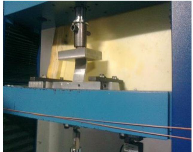
Fig-4: Experimental setup of buckling by using UTM.
