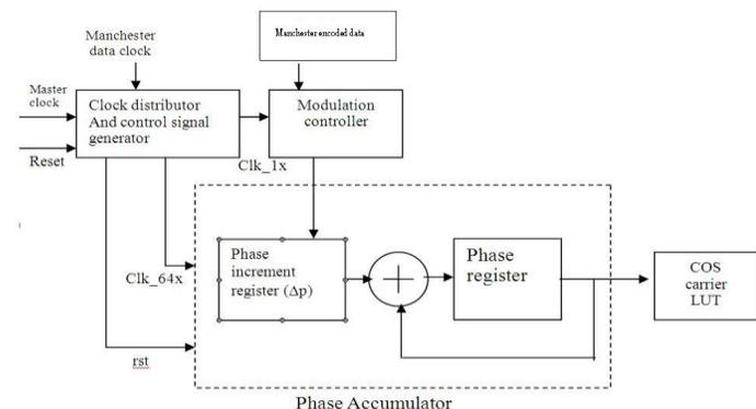
Fig 4. Direct digital synthesizer for Carrier generation
