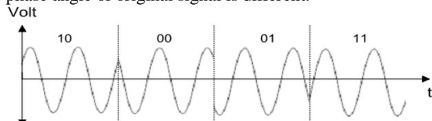
Fig. 2 Output waveform of QPSK modulator i.e., SQPSK
