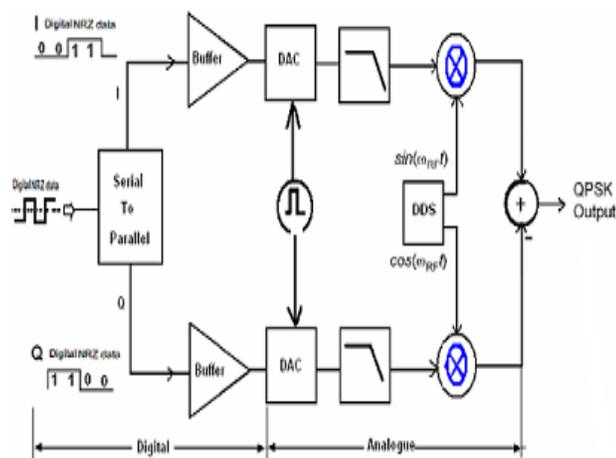
Fig. 1 Conventional QPSK Modulator
