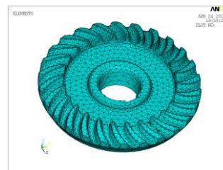
Fig. 7.shows the Finite element model of the crown wheel gear
