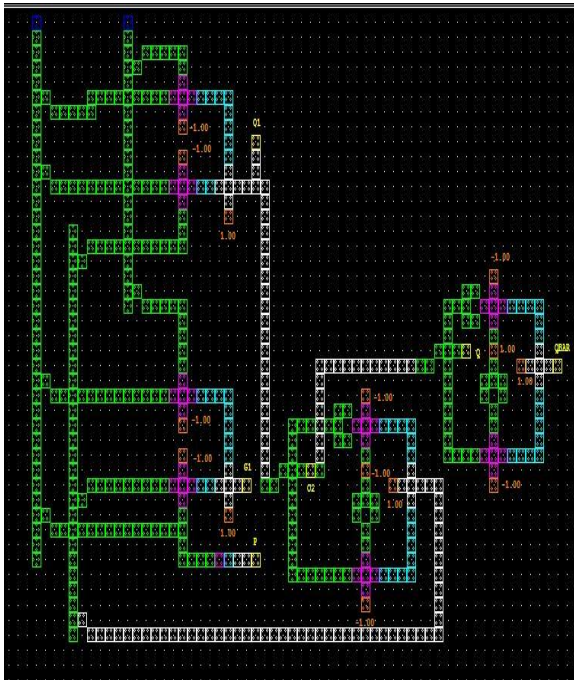
Fig 8.QCA layout for Fredkin-Feynman based D-latch with output Q and Q'.
