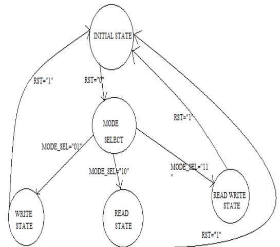
Fig.3. State diagram for Memory mode selection
