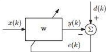
Fig .2. Basic Diagram of Adaptive filter
