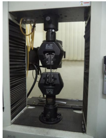
Fig. 4 Specimen subjected to Tension Test on UTM.
