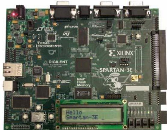
Fig. 3 Spartan 3E FPGA board
