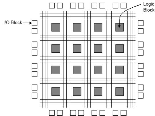
Fig. 4 FPGA structure
