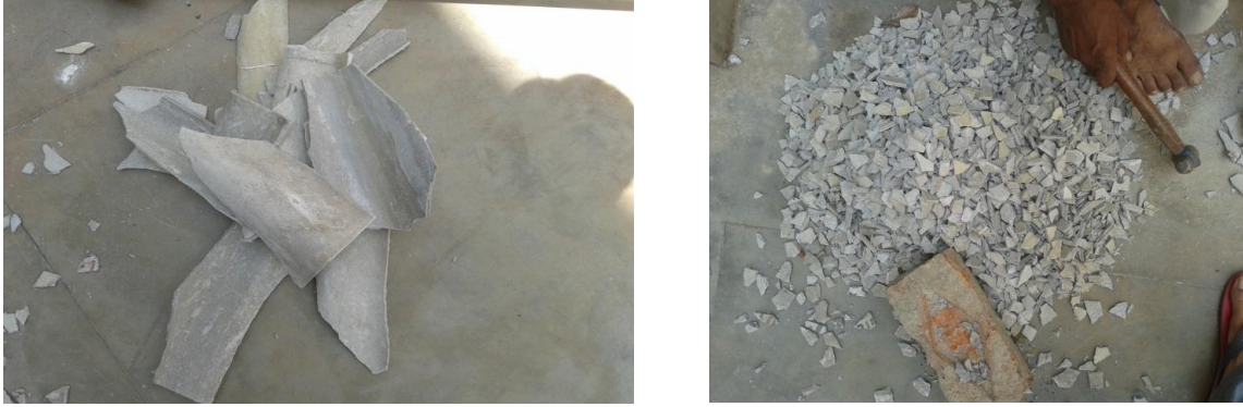
Fig. 2 Breaking of Asbestos Cement Sheet Waste into pieces by hammer
