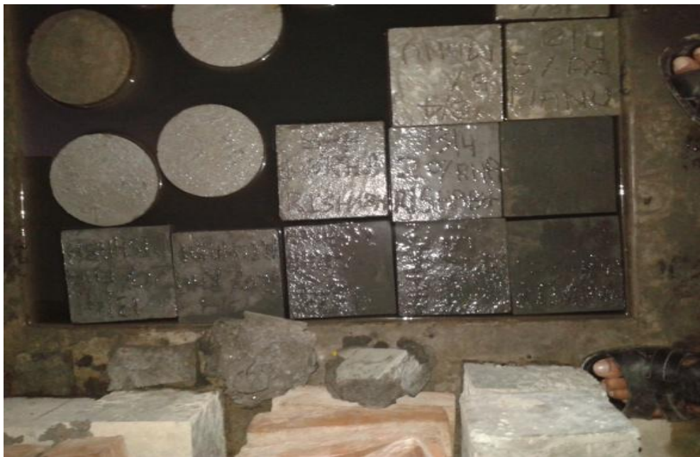
Fig. 7 Curing of Cubes
