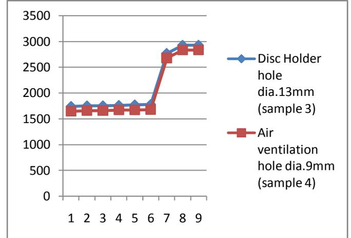
**Graph** Effect of increased air ventilation hole diameter on natural frequency of brake disc.
