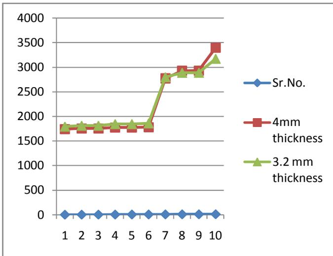
**Graph** Effect of wear of brake disc on FEM natural frequency.
