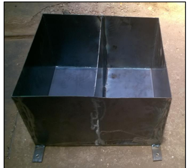
Fig. 2 Oil tank divided in two chambers
