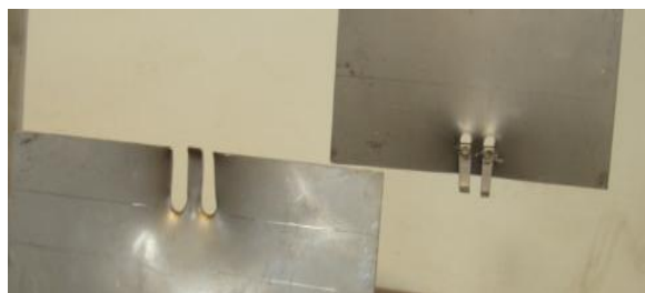
Fig.6 .Pull out failure mode
