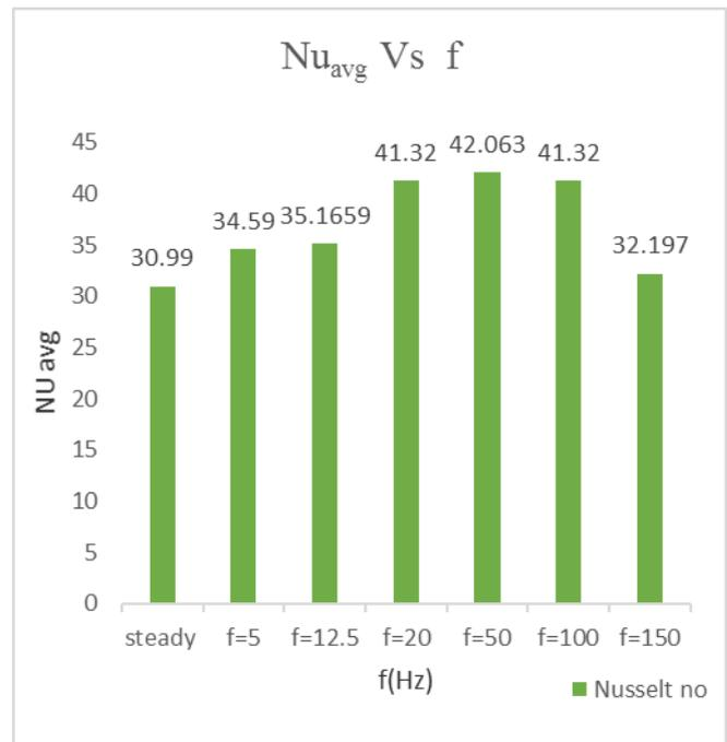
Fig.4.1Variation of average Nusselt number for steady and pulsed jet with different frequencies at Re=5000 and Z/D=3
