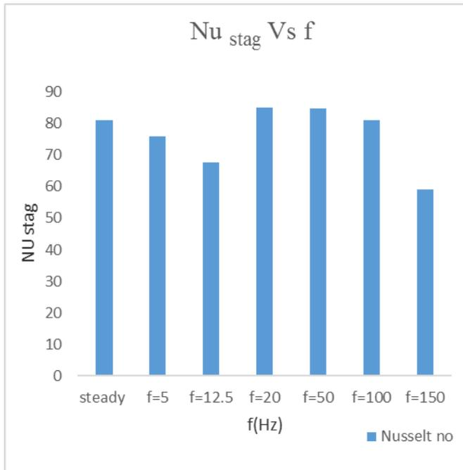
Fig. 4.2 Variation of stagnation Nusselt number for steady and pulsed jet with frequency at Re=5000 and Z/D=3
