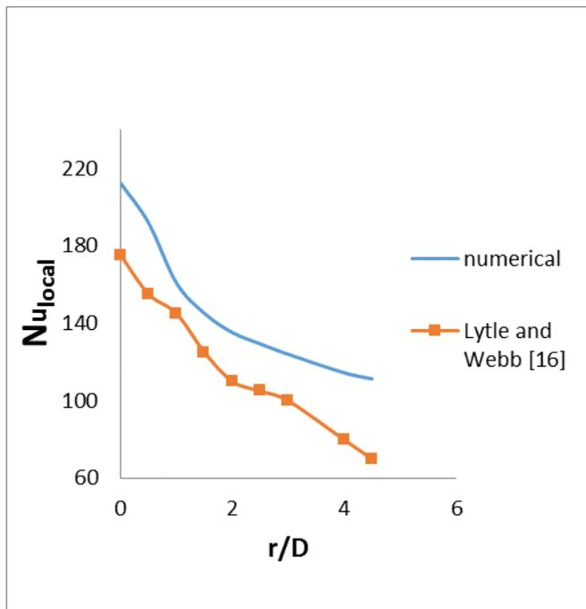
Fig.4.Variation of Local Nusselt number with radial distance for Re=23000, Z/D=6
