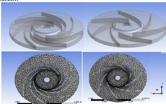
Figure 2.5 Geometry and meshed models
