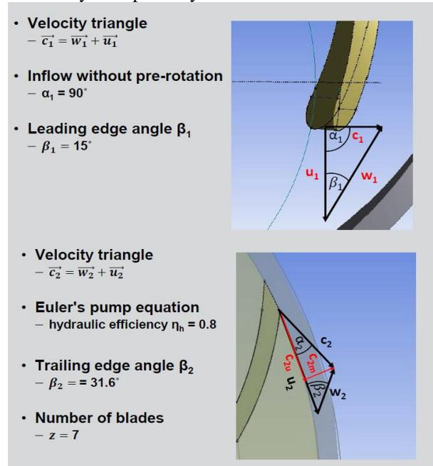
Figure 2.3 Velocity triangles at inlet and outlet
