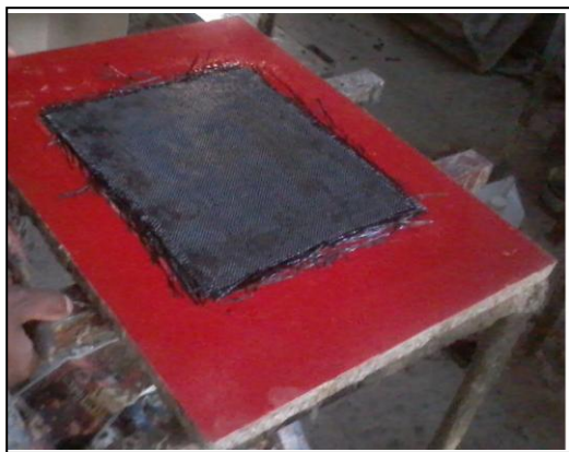
Fig-1: Wood mould used for hand lay up technique
