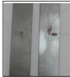
Fig.4.1 MS Plate without strain gauge and Plate with two strain gauge rosette
