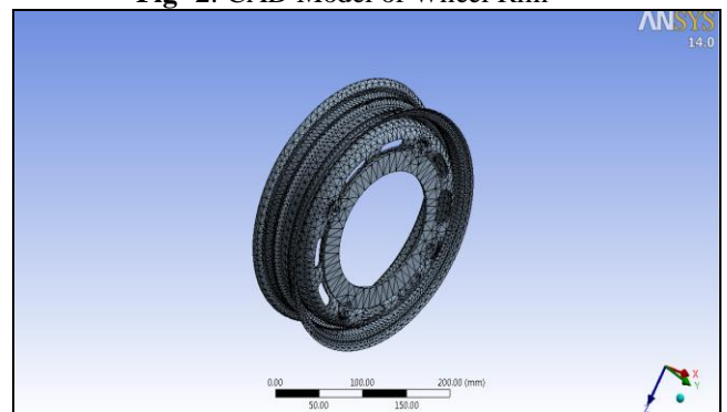
Fig -3: Meshing of wheel rim (10 Node Tetrahedron Element)
